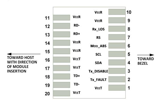
**Host PCB SFP Pad Assignment Top View**
